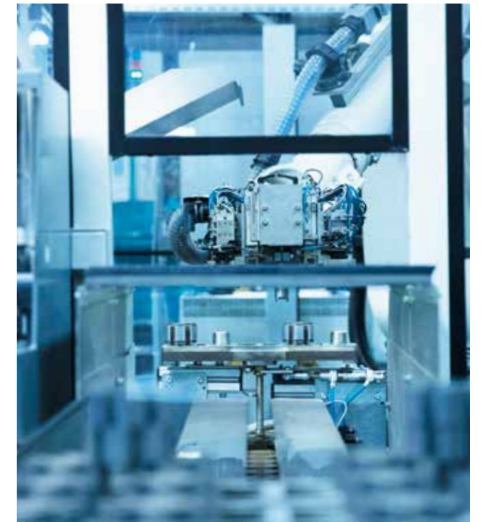
Metal and plastic joining: in-tool stacked components ready for assembly with plastic insulation.
