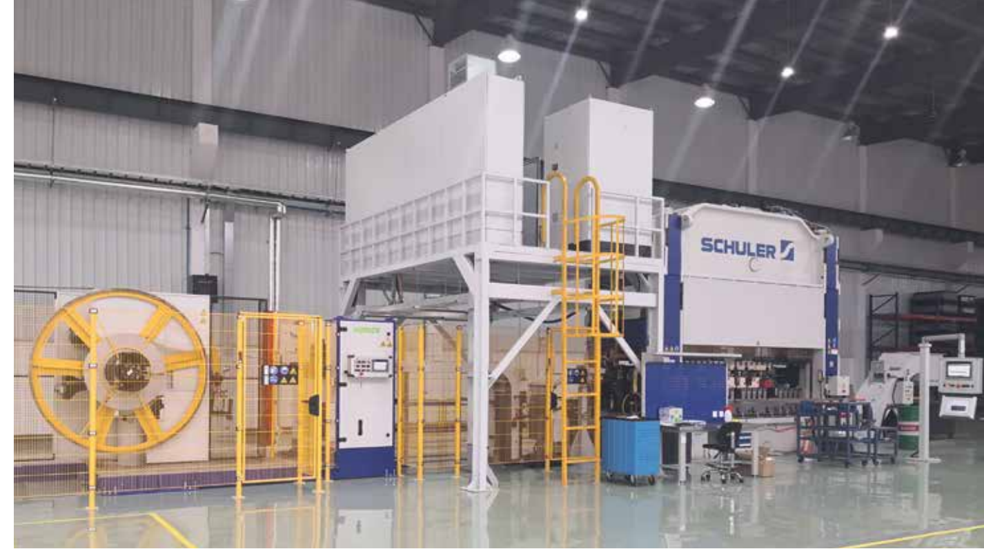
Cutting-edge high-speed blanking presses ensure that production at the plant in Taicang, CN, is cost-effective.
