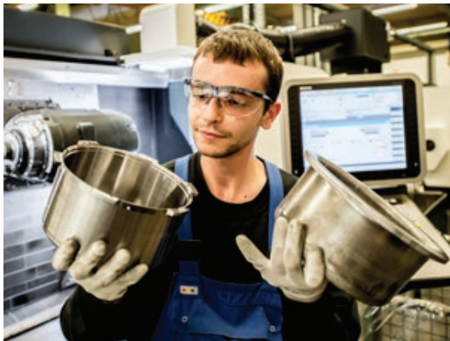
Hybrid components: multiple deep-drawing operations and machined on a CNC turning and milling center
