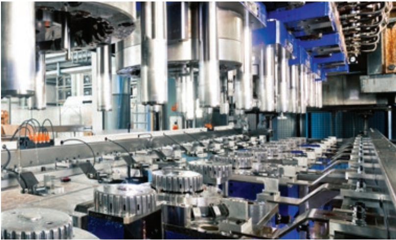
Transfer press: volume production of clutch disc carriers in a twelve-station roller tooling configuration
