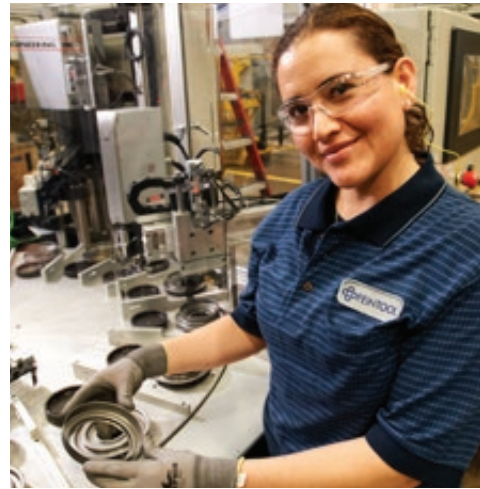
Piston assembly including dimensional checks, leak testing and laser marking
