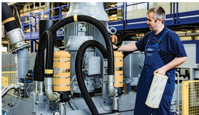
Prompt intervention: Thanks to FEINmonitoring, the oil filter of a press is changed promptly and unplanned downtimes are avoided.
