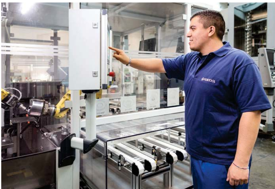
At the push of a button. The deburring unit operates almost entirely automatically.
