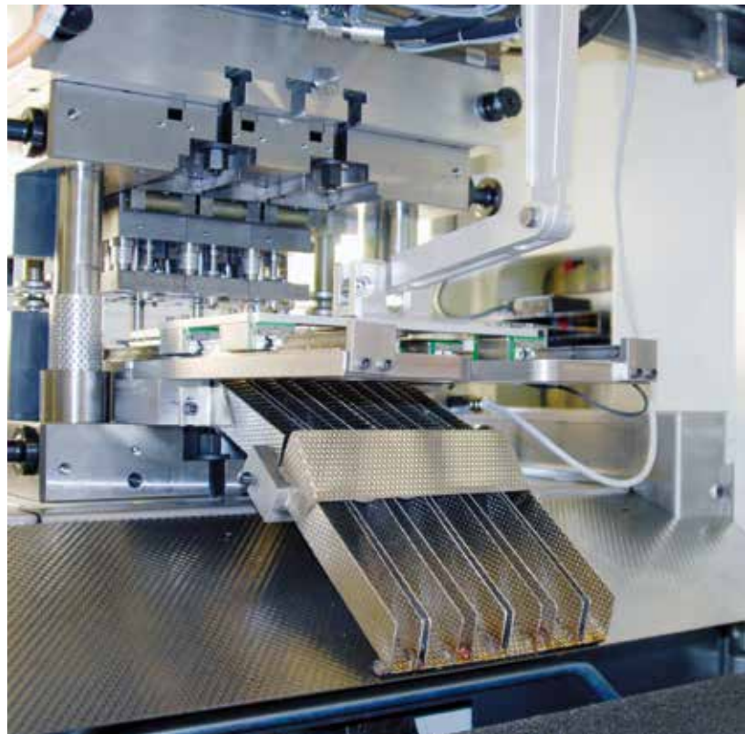
The removal device is integrated into the press control system to ensure damage-free part removal
