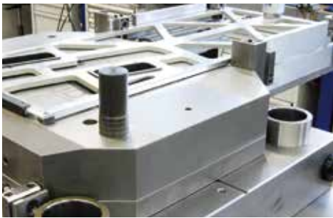
Slider plate for controlled parts removal
