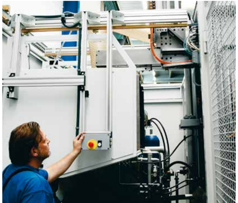
Integrated removal system for simple changeover from compressed air ejection to parts removal
