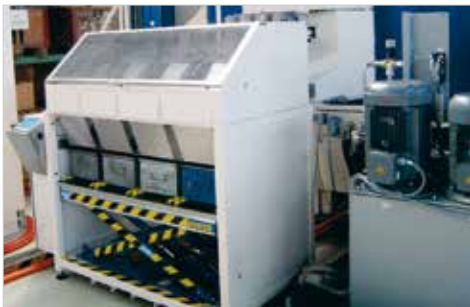
Filling station for separated four-track transfer of parts to downstream processing
