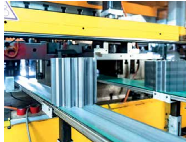
In-tool stacked rotor and stator cores
