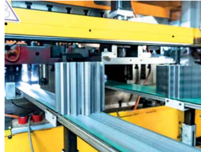
Interlocked rotor and stator cores
